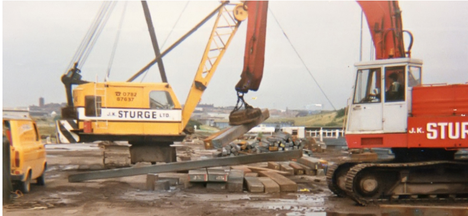
Figure 11.1.1: An industrial electromagnet is capable of lifting thousands of pounds of metallic waste. (credit: modification of work by "BedfordAI"/Flickr)
