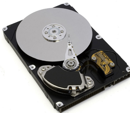
Figure 12.8.6: The inside of a hard disk drive. The silver disk contains the information, whereas the thin stylus on top of the disk reads and writes information to the disk.
