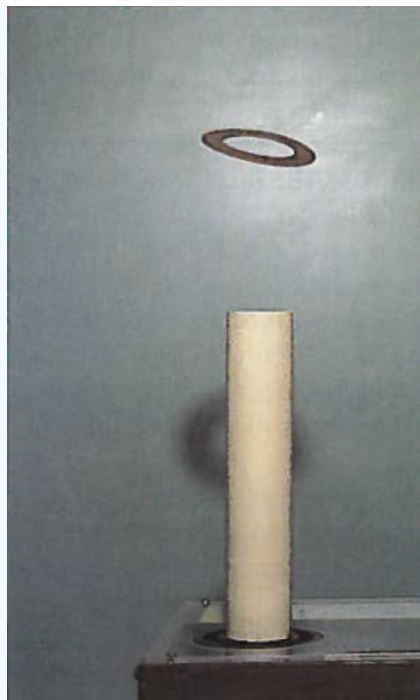
Figure 13.3.4: The jumping ring. When a current is turned on in the vertical solenoid, a current is induced in the metal ring. The stray field produced by the solenoid causes the ring to jump off the solenoid.
