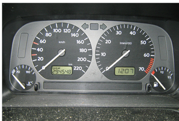
Figure 10.5.1: The fuel and temperature gauges (far right and far left, respectively) in this 1996 Volkswagen are voltmeters that register the voltage output of “sender” units. These units are proportional to the amount of gasoline in the tank and to the engine temperature. (credit: Christian Giersing)
