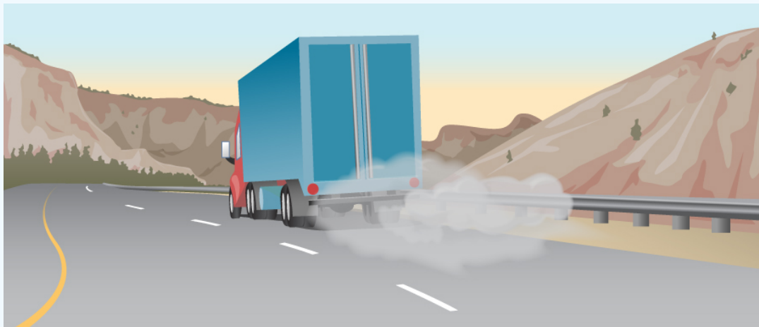
Figure 1.5.3: The smoking brakes on a braking truck are visible evidence of the mechanical equivalent of heat.
