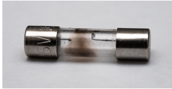
Figure 9.6.3: A fuse consists of a piece of wire between two contacts. When a current passes through the wire that is greater than the rated current, the wire melts, breaking the connection. Pictured is a “blown” fuse where the wire broke protecting a circuit (credit: modification of work by “Shardayy”/Flickr).
