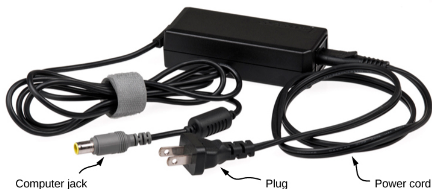
Figure 5.3.1: This power adapter uses metal wires and connectors to conduct electricity from the wall socket to a laptop computer. The conducting wires allow electrons to move freely through the cables, which are shielded by rubber and plastic. These materials act as insulators that don't allow electric charge to escape outward. (credit: modification of work by "Evan-Amos"/Wikimedia Commons)
