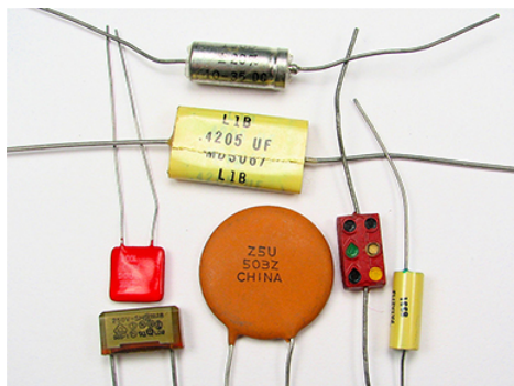
Figure 8.2.3: These are some typical capacitors used in electronic devices. A capacitor's size is not necessarily related to its capacitance value.
