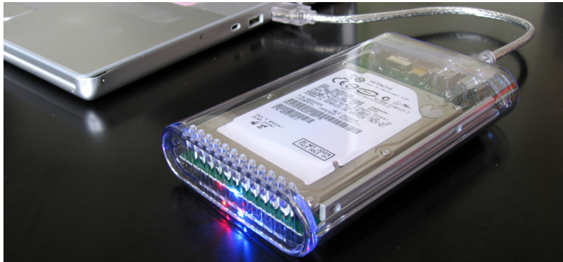
Figure 12.1.1: An external hard drive attached to a computer works by magnetically encoding information that can be stored or retrieved quickly. A key idea in the development of digital devices is the ability to produce and use magnetic fields in this way. (credit: modification of work by “Miss Karen”/Flickr)
