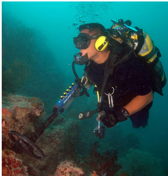
Figure 15.6.3: When a metal detector comes near a piece of metal, the self-inductance of one of its coils changes. This causes a shift in the resonant frequency of a circuit containing the coil. That shift is detected by the circuitry and transmitted to the diver by means of the headphones.
