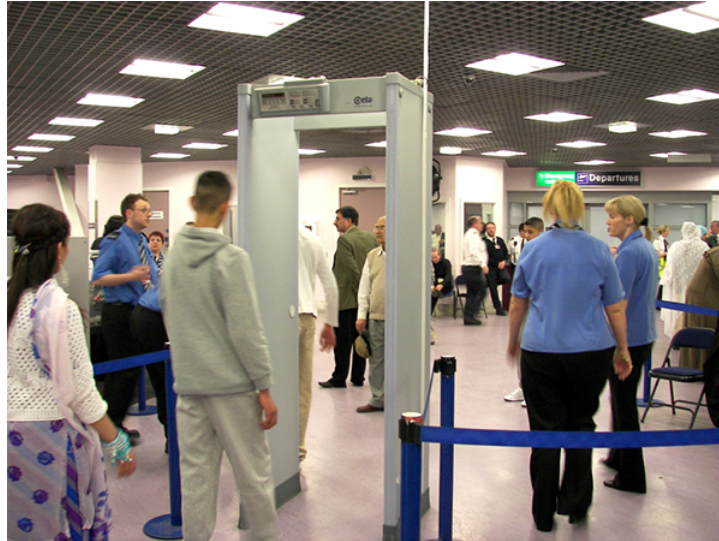
Figure 14.3.5: The familiar security gate at an airport not only detects metals, but can also indicate their approximate height above the floor. (credit: “Alexbairds”/Wikimedia Commons)
