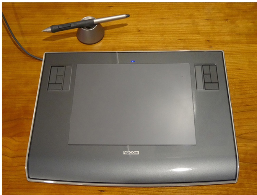
Figure 13.8.1: A tablet with a specially designed pen to write with is another application of magnetic induction.
