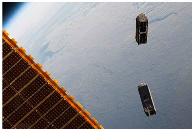
Figure 16.5.3: Two small CubeSat satellites deployed from the International Space Station in May, 2016. The solar sails open out when the CubeSats are far enough away from the Station.
