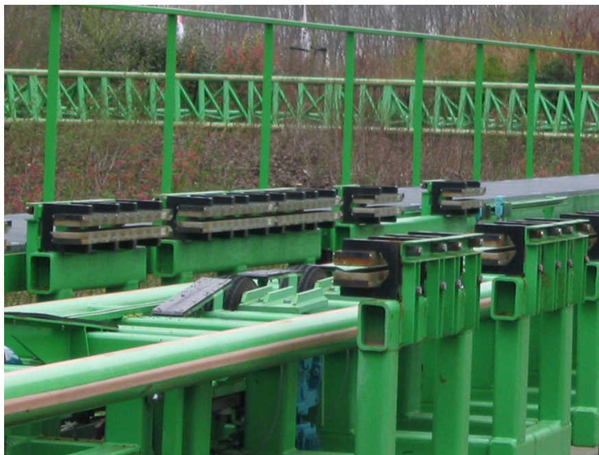
Figure 13.6.7: The rows of rare-earth magnets (protruding horizontally) are used for magnetic braking in roller coasters. (credit: Stefan Scheer)
