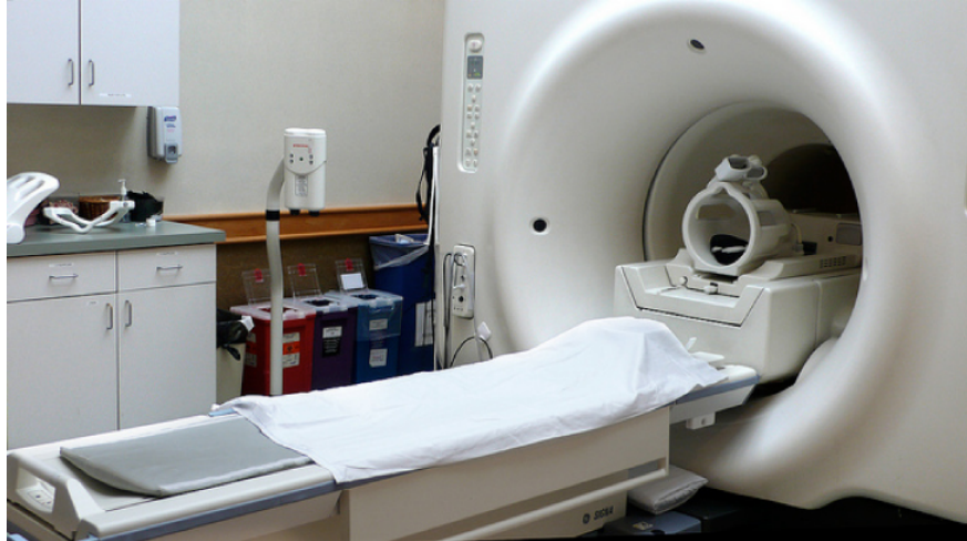
Figure 12.7.3: . In an MRI machine, a large magnetic field is generated by the cylindrical solenoid surrounding the patient. (credit: Liz West)
