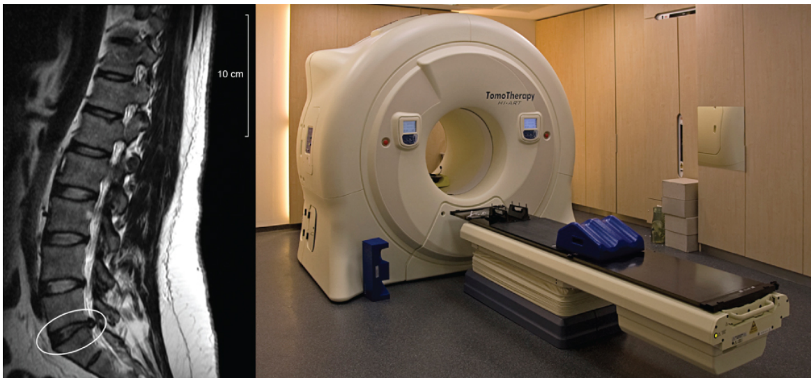
Figure 9.1.1: Magnetic resonance imaging (MRI) uses superconducting magnets and produces high-resolution images without the danger of radiation. The image on the left shows the spacing of vertebrae along a human spinal column, with the circle indicating where the vertebrae are too close due to a ruptured disc. On the right is a picture of the MRI instrument, which surrounds the patient on all sides. A large amount of electrical current is required to operate the electromagnets (credit right: modification of work by "digital cat"/Flickr).
