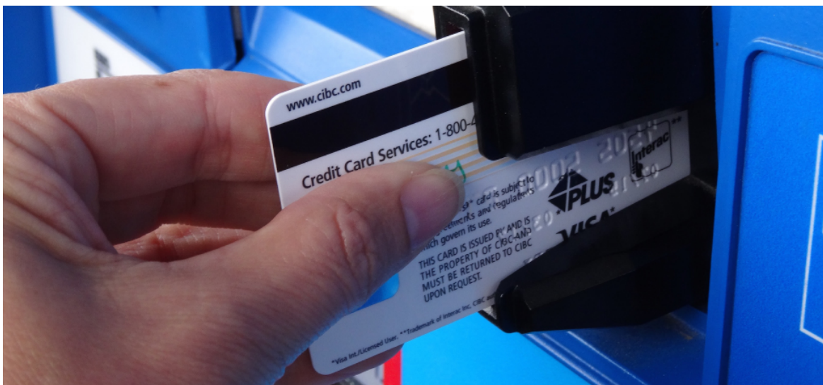
Figure 13.1.1: The black strip found on the back of credit cards and driver's licenses is a very thin layer of magnetic material with information stored on it. Reading and writing the information on the credit card is done with a swiping motion. The physical reason why this is necessary is called electromagnetic induction and is discussed in this chapter.
