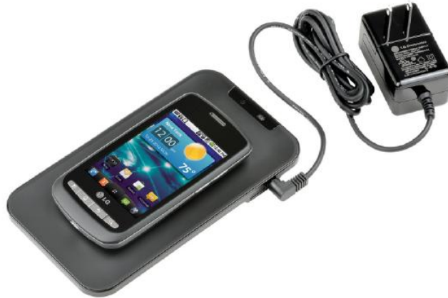
Figure 14.1.1: A smartphone charging mat contains a coil that receives alternating current, or current that is constantly increasing and decreasing. The varying current induces an emf in the smartphone, which charges its battery. Note that the black box containing the electrical plug also contains a transformer (discussed in Alternating-Current Circuits ) that modifies the current from the outlet to suit the needs of the smartphone. (credit: modification of work by “LG”/Flickr)
